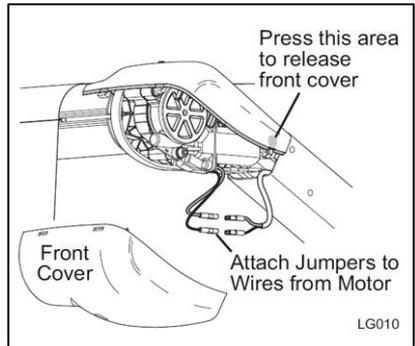
5. When the awning is closed, remove the jumper wires and reattach the cable wires to the motor wires. Be sure to match RED to RED and BLACK to BLACK.
