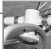
**NOTE:** In the Water Heater Bypass Diagram, valve D is the fresh water tank shutoff. Valve E is used to introduce RV antifreeze into the lines when winterizing the system and has a clear hose attached to it. See Winterizing the Plumbing System in this manual. Valves D & E are typically located in the vicinity of the water pump which can be under a dinette bench, kitchen island, or bed.
