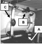
Factory installed water heater bypass
