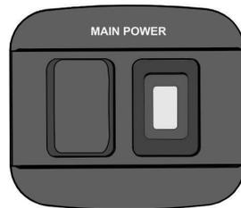
**longer than 1 second. Depressing and holding the switch down will disable the battery disconnect solenoid.** Should this occur the main ground cable for the house batteries must be removed for 1 minute to re-enable the solenoid operation.
