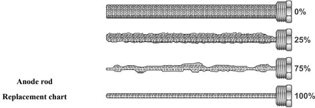
Operating the water heater without the proper anode rod protection will decrease tank life and will void the tank manufacturer's warranty on the tank. To extend the anode life, drain the water from the water heater tank whenever the motor home is not being used. Avoid any extended time of non-use with water in the tank.
